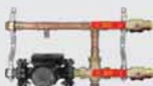
Mixing station Base unit - For supply temperature modulation - Equipped with circulator Model 2801.1US, 2801.9US Components Isolation ball valves, mounting bracket, supply temperature sensor well, 3-speed circulator Model 2801.0US
