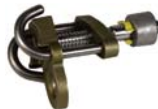
Wire Grip Grips conductor, has hole for block or line hook. WWL for grip is 1,000 lbs (454 kgs) at a 4:1 ratio. 3600 Opening min.5/16" max.7/8" 2 lbs (0.91 kgs) (7.9mm, 2.2cm) 3601 Opening min.1/2" max.1-1/2" 3 lbs (1.36 kgs) (1.3cm, 3.8cm) Add suffix "U" for Universal, "Q" for Quick Change
