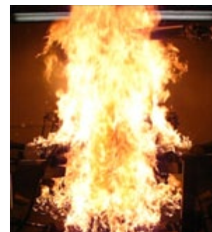
A simulated flash fire on an FR garment.
