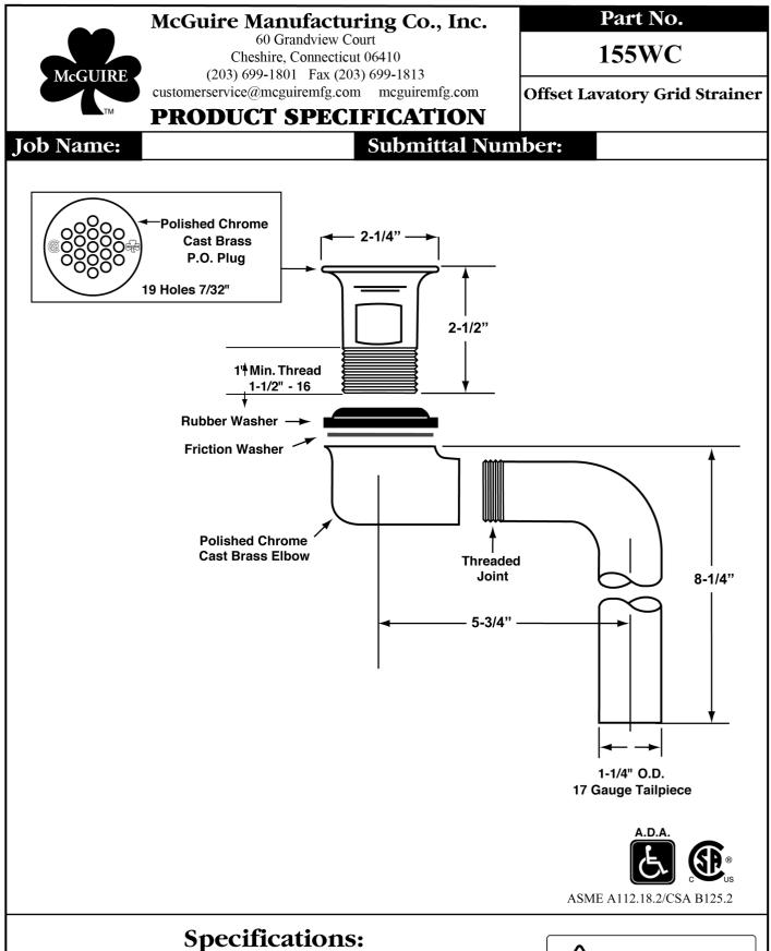
Cast brass chrome plated offset wheelchair strainer with polished chrome cast brass elbow, 17GA 1-1/4" seamless brass offset tailpiece, rubber basin washer and fiber friction washer. Offset lavatory strainer shall be in compliance with CSA or other recognized testing authority and bear both manufacturer and testing mark.
