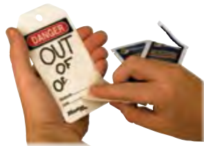
Wipe off current message with Isopropyl Alcohol
