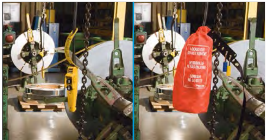
Hoist Control Cover
