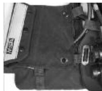
6. Insert the right tri-bar of the rescue belt into the outer right slot of the back plate.
