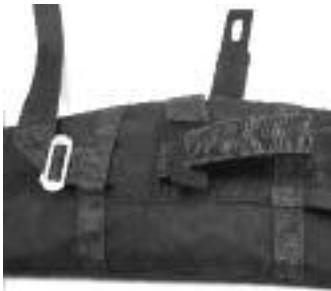
7. Pull the tri-bar to the left until the sewn fold in the quick release-strap has been pulled tight against the left slot in the Nomex plate.
