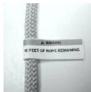
5. Verify that the releasable termination knot is at the end of the rope and that all labels are in place.
