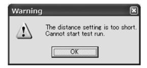
Fig. 13.54 Operation Unable Message due to Moving Distance too short
